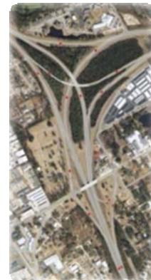
The public identified the interchanges of SC 9 at US 17 and Sea Mountain Highway at US 17 as confusing and dangerous. Reconfiguration of SC 9 at US 17 will include the addition of two movements through the construction of new ramps. At the interchange of Sea Mountain Highway and US 17, the dangerous and confusing weave section was eliminated by realigning minor movements to Sea Mountain Highway.
