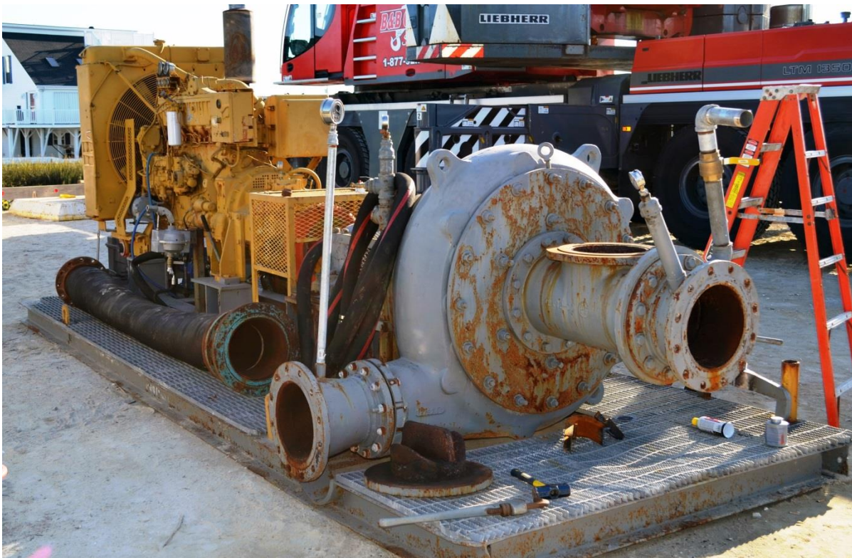
A booster pump will be launched on a small barge to ensure a steady flow of dredged materials through the pipeline to the spoils basin.
